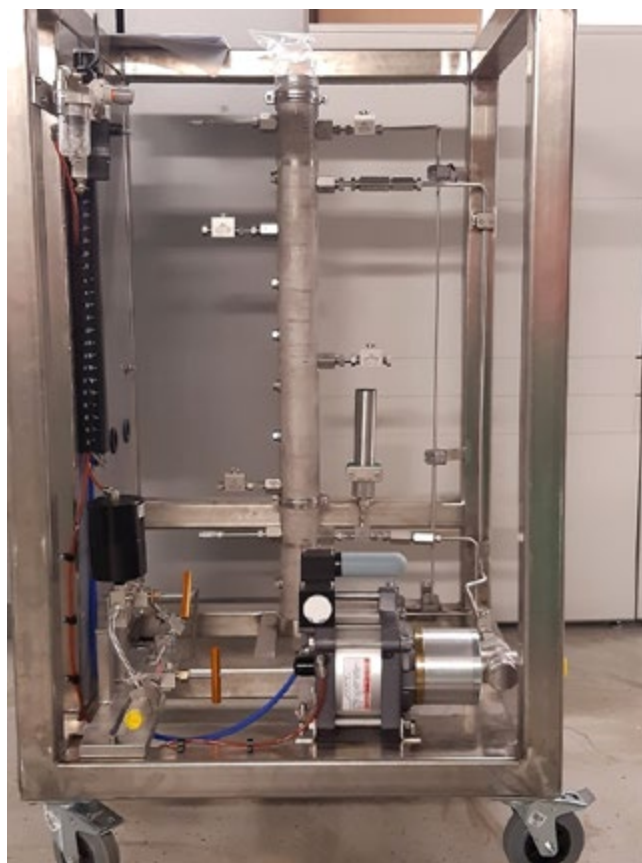
Figure 5.1. Continuously operating reactor developed for carbon dioxide extraction (Photo: Petri Österberg, Oulu University).
