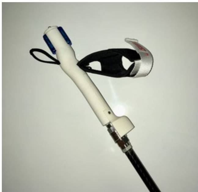
Figure 8.2. A pole force sensor in the HYTELI project.
