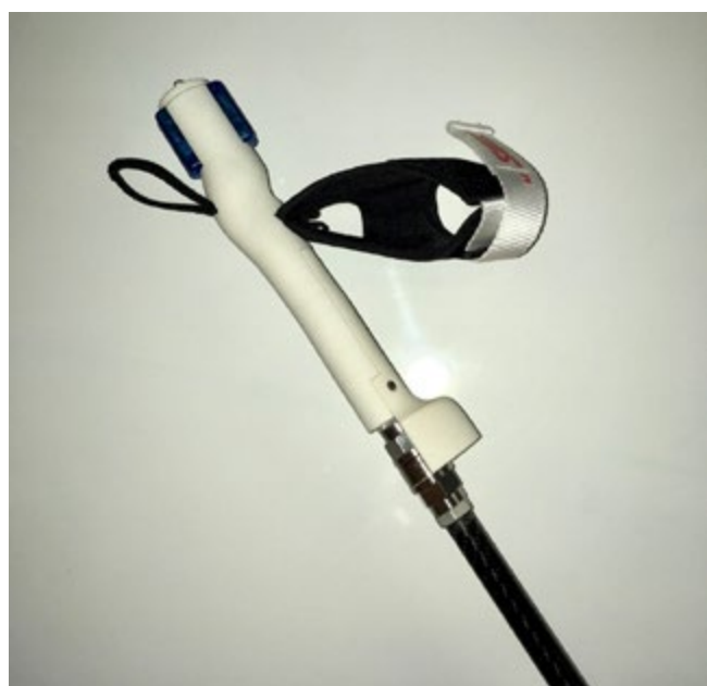
Figure 5.4. A pole force sensor in the HYTELI project
