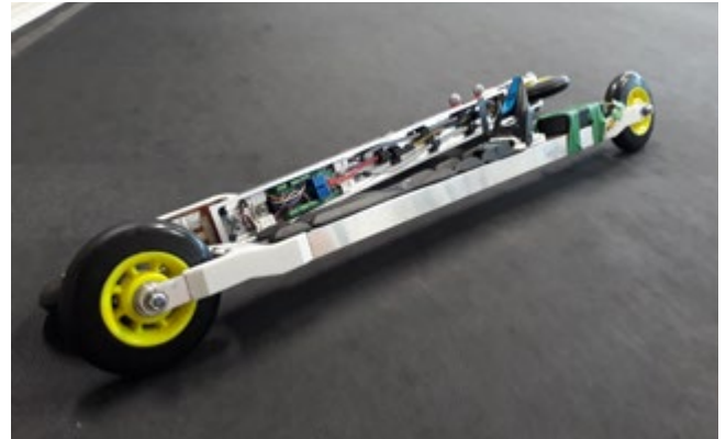
Figure 8.2. Roller ski sensors and ski pole force sensors implemented in HYTELI project.
