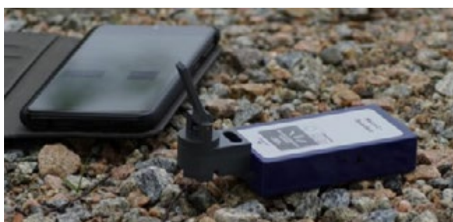
Figure 4.3. A measurement device for nickel measurement was developed in MINIME project.
