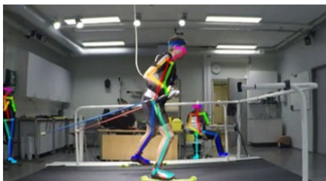
Figure 9.2. In HYTELI project, CSC developed further human pose estimation methods for dynamic balance tests and treadmill skiing.
