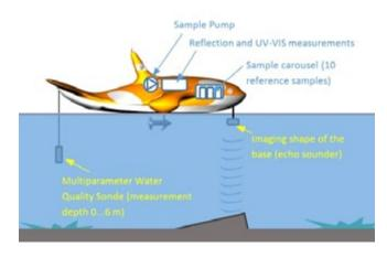
Figure 4.5. The KAIMIT project used the MITY water measurement vessel for sample collection and measuring.
