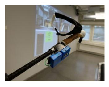
Figure 4.6. Prototype sensing using a piezoelectric sensor to measure ski pole forces, with the force sensor fastened between the pole and the handle.
