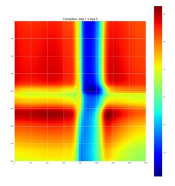
Figure 4.4. Visualisation of cross-correlation analysis of NIR sensor data from two-line wavelength data. Based on the analysis, it was possible to determine the delay between the lines.
