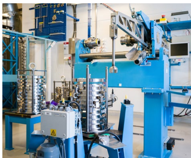
Picture 7.1. The VTT MIKES 2 kNm torque standard for calibrating torque sensors is located in Kajaani.
