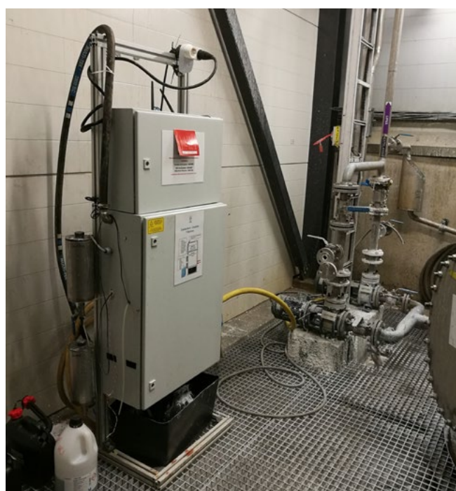
Picture 4.1. The real-time NIR measuring device developed by MITY in the industrial pilot test.
