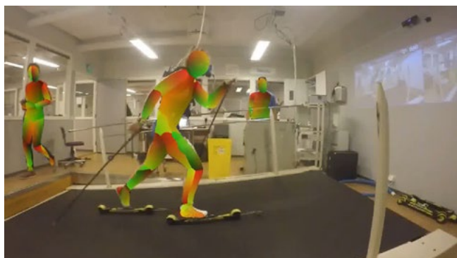
Picture 9.2. Various neural network models for recognising the posture of an athlete have been trialed in the context of the LIIKUTPA project.
